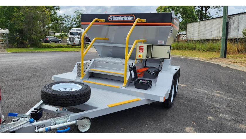
The SP1000 is a simple-to-use, tandem-axel binder spreader trailer purpose-built for insitu stabilization. This trailer is cost-effective because it is accurate and has proven capable of consistent spread rates of plus or minus 10%
