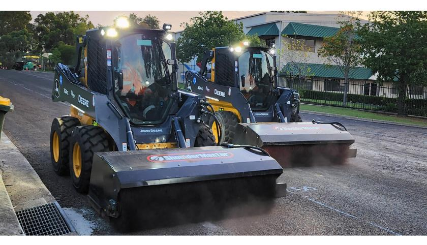
The ShoulderMaster Bucket Broom is a tough, reliable, and easy-to-use open-face broom. It features a large collection bucket with bolt-on wear plates for easy maintenance. The brush is adjusted with an easy and quick 4-stage adjuster bolt with total brush replacement exchanged by a one-piece poly brush for easy on-site maintenance.
